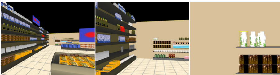
Figure 3.9: Continuous Zoom progressive refinement technique: the user can continuously zoom towards the pointed direction. (BACIM; KOPPER; BOWMAN, 2013)
