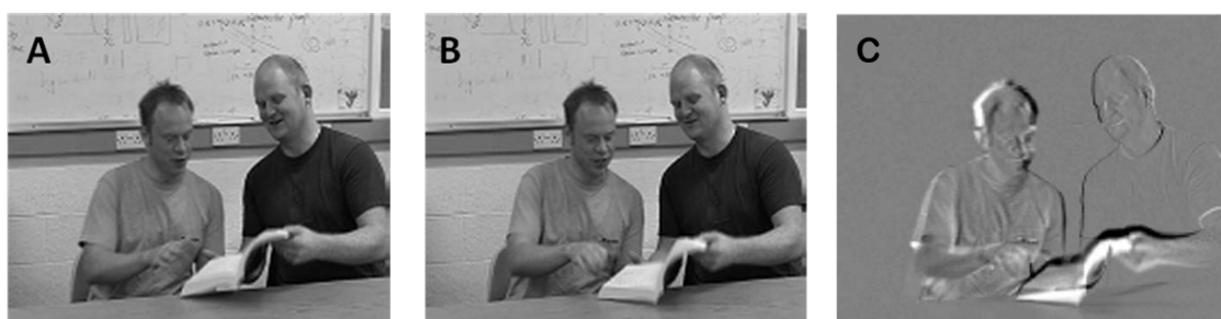
Figure 2.8 – (A) and (B) show consecutive frames, while (C) shows the residual difference between (A) and (B) frames.
